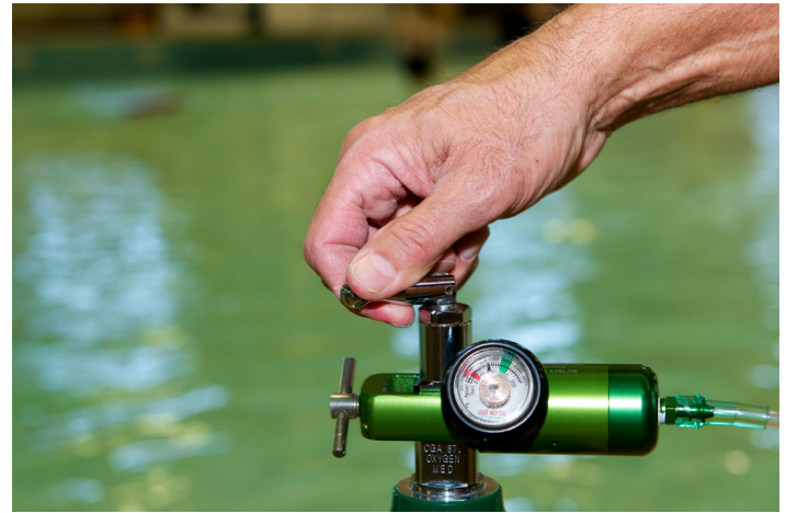
Figure 1.5 With the cylinder opened the pressure gauge reflects the amount of pressure in the cylinder.
