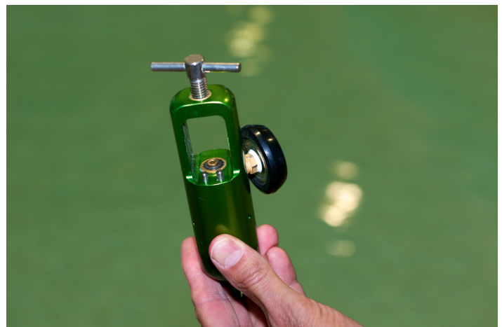
Figure 1.4 An oxygen pressure regulator has unique metal prongs that engage matching holes of the oxygen cylinder.
