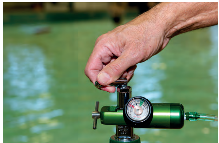
Figure 12.5 With the cylinder opened the pressure gauge reflects the amount of pressure in the cylinder.
