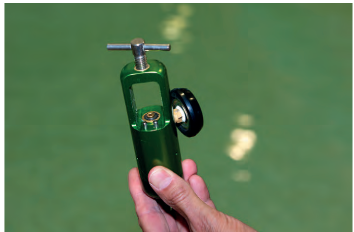
Figure 12.4 An oxygen pressure regulator has unique metal prongs that engage matching holes of the oxygen cylinder.
