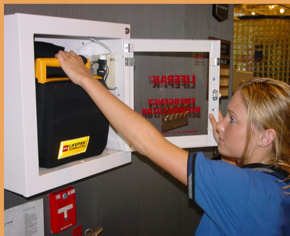
AEDs run internal diagnostics to ensure proper working condition. Warning lights verify for users that the device is ready.
