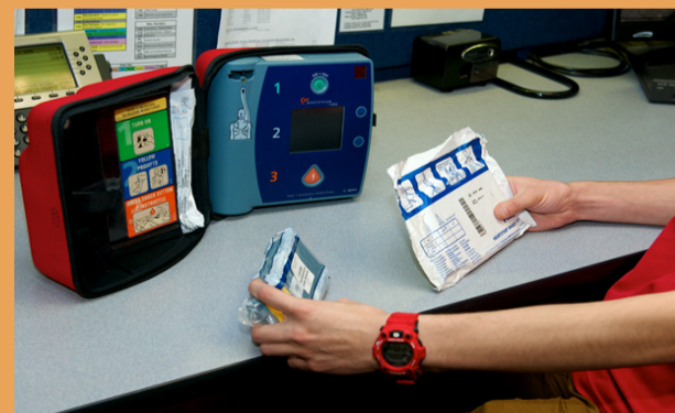
Periodic inspection of the AED will ensure it is proper function and that the necessary supplies are available and up-to-date.
